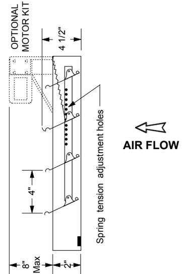
**CAUTION:** Motor kits are not suitable for use in explosive or flammable areas or airflows.
